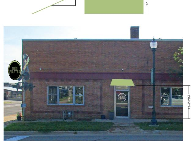
AWNINGS & PROJECTION SIGN TO BE INSTALLED WITH WEJ-IT ANCHORS AND EPOXY IF NEEDED
