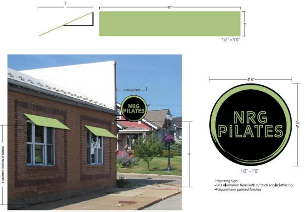
PMS 577 AWNINGS & PROJECTION SIGN TO BE INSTALLED WITH WEJ-IT ANCHORS AND EPOXY IF NEEDED
