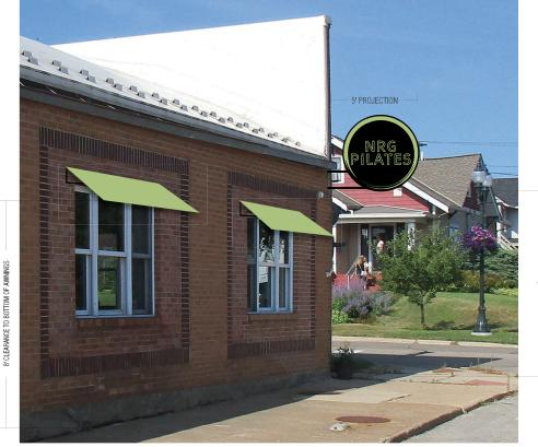
PMS 577 AWNINGS & PROJECTION SIGN TO BE INSTALLED WITH WEJ-IT ANCHORS AND EPOXY IF NEEDED
