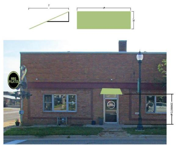
AWNINGS & PROJECTION SIGN TO BE INSTALLED WITH WEJ-IT ANCHORS AND EPOXY IF NEEDED
